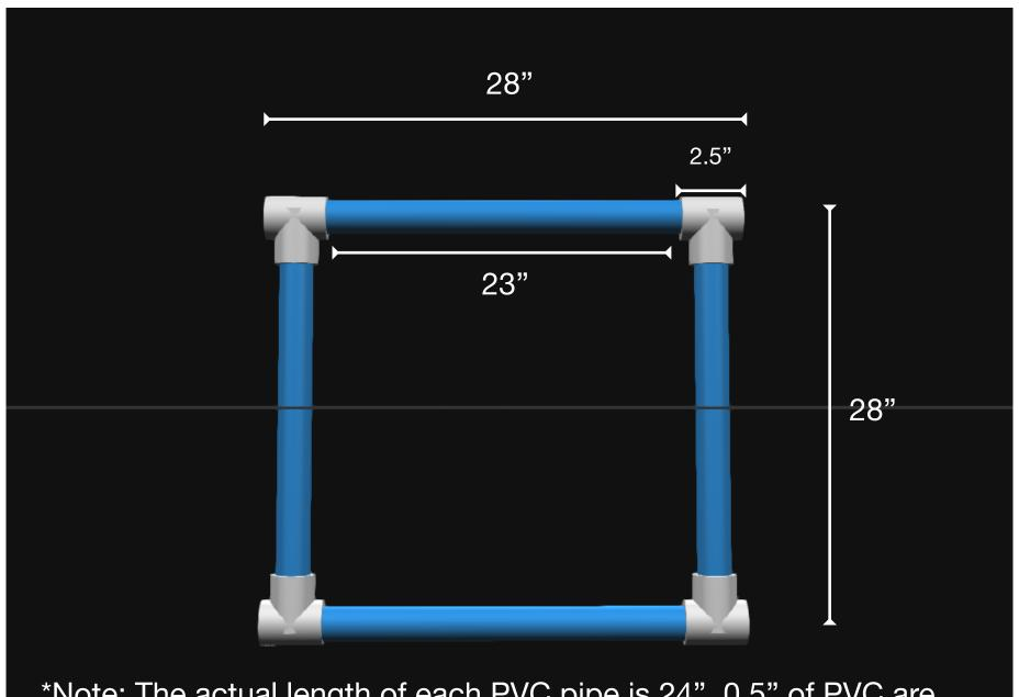
\*Note: The actual length of each PVC pipe is 24". 0.5" of PVC are inserted into each T-adapter.
